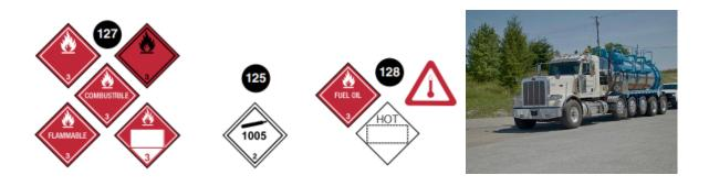
This is driven by DOT FMCSA. Pun intended. DOT 406/407 (formerly designated MC307 and MC312) and 412 for vacuum trucks list the requirements for coded vessels.
